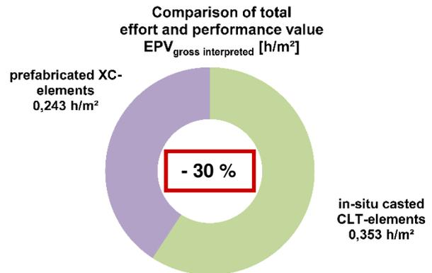
**Figure 11:** Comparison of EPV – EPV for different tasks included in the in-situ variant (upper graph), total EPV for the installation of the systems (lower graph) [1]
