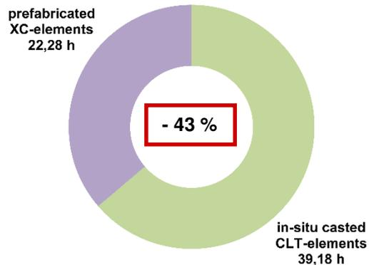
Figure 7: Comparison of building times for both variants – number of working time required for different activities (upper graph), summation of working time required (lower graph) [1]
