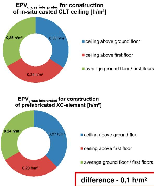
**Figure 10:** Total EPV<sub>gross interpreted</sub> – EPV for different ceilings and on average of the in-situ variant (upper graph), and prefabricated XC-variant (lower graph) [1]
