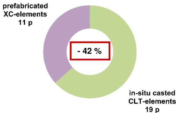
Figure 8: Comparison of workforce involved – number of workers required for different activities (upper graph), summation of all workers required (lower graph) [1]
